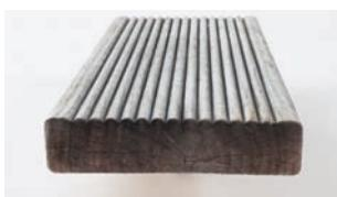
Swedish OrganoWood is a modified timber where naturally occurring silicon is bonded to wood fibres under high pressure to partially fossilise them.
