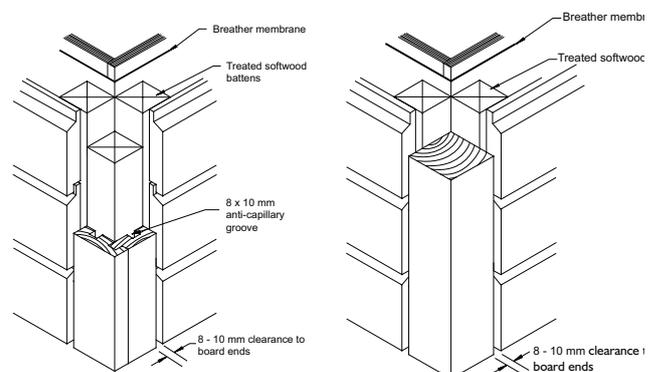
Mitreing boards at corners is not recommended, as natural movement of the timber will allow the joint to open, causing failure of the surface coating and water ingress. Mitreing the ends of boards can be considered, but it is advisable to provide a gap between any adjoining surfaces.
